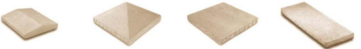
PEAKED WALL CAPS Available in 2 sizes: 20" × 16" (2"H sides with a 3.5"H peak) 20" × 12" (2.375"H sides with a 3.5"H peak) TEXTURED COLUMN CAPS Cap peak approx. 5.5"H. Available in 3 sizes with or without hole: 26" × 26" (2.5"H sides) 22" × 22" (2.5"H sides) 18" × 18" (2.5"H sides) COLUMN CAPS Column Caps approx. 2.5" thick. Available in 2 sizes: 30" × 24" 24" × 24" WALL CAPS Wall Caps approx. 2.25" thick. Available in 3 sizes: 37" × 12" 37" × 9" 37" × 6"
